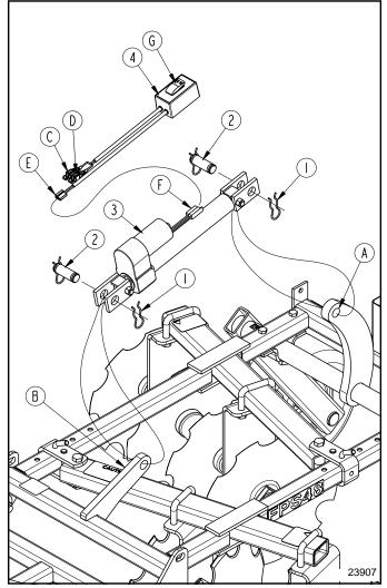
Linear Actuator Assembly () Figure 1-1
